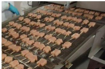
The stick inserter can be provided with different conveyors to ensure that the satay is not cooked in the fryer against each other. This helps to avoid white spots on the satay and satay which is not cooked.
