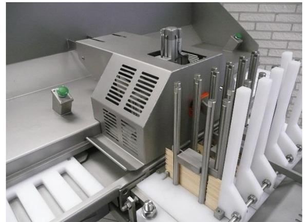
The machine is simple and rapid change of stick length. Also, the form plates are easily to change. As a result, for example, you can switch from four pieces meat 180mm to two pieces on a 100 mm stick length. The machine can run approximately 15 strokes per minute, depending on the number of products on a stick and staff that the machine is using. In each stroke 8 sticks are pushed into the products.
