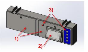
push-buttons for the most common operations (see picture No. 3). The rest is regulated through the Touch Panel. The Touch Panel is secured by means of an additional viewing window for cleaning the machine.
